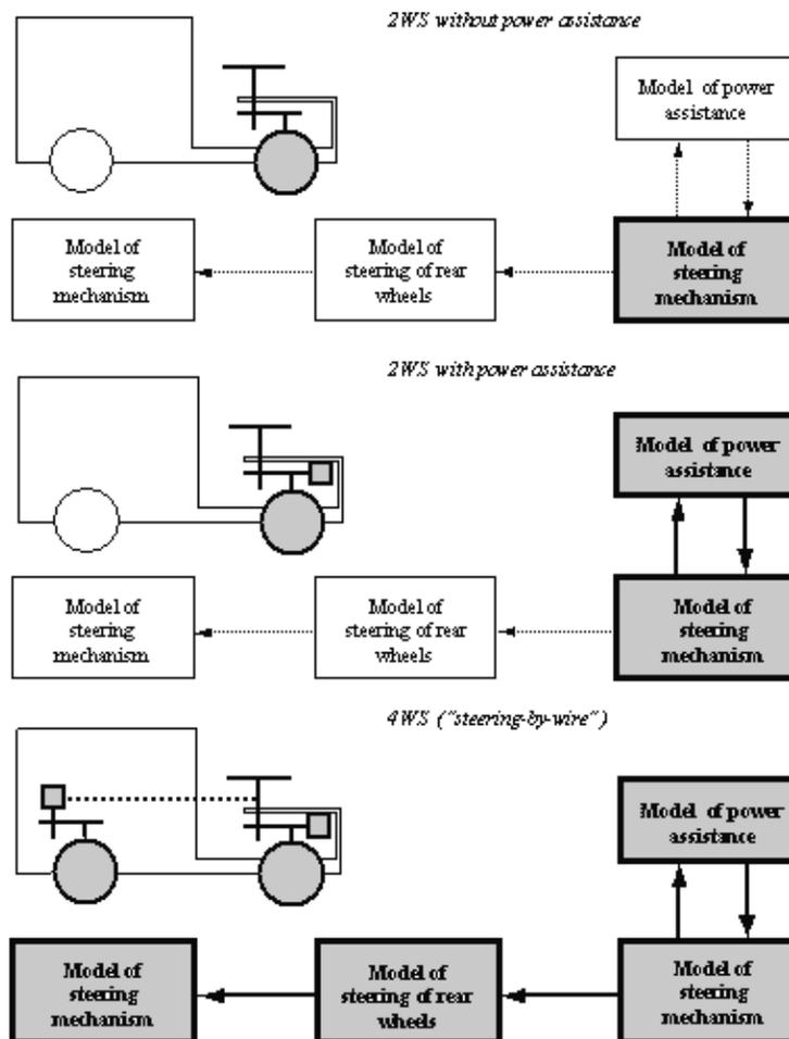
Fig. 7. Idea of modular form of steering system model
