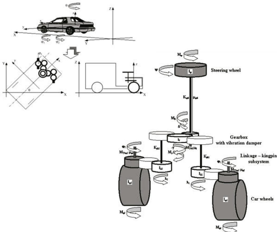
Fig. 6. Idea of substitutive physical model of steering system mechanism
