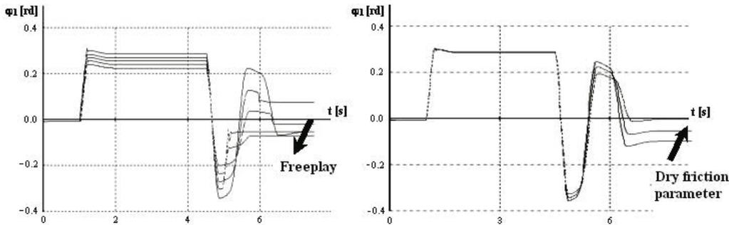
Fig. 8. Example simulation results (time history of left wheel angle) for combined ISO road test of 2WS car with steering system without power assistance. Dry friction parameter  $M_{T\phi 0} \in [1.35, 4.05] \text{Nm}$ , freeplay parameter  $(\delta-p\gamma)_0 \in [0, 0.27] \text{rd}$
