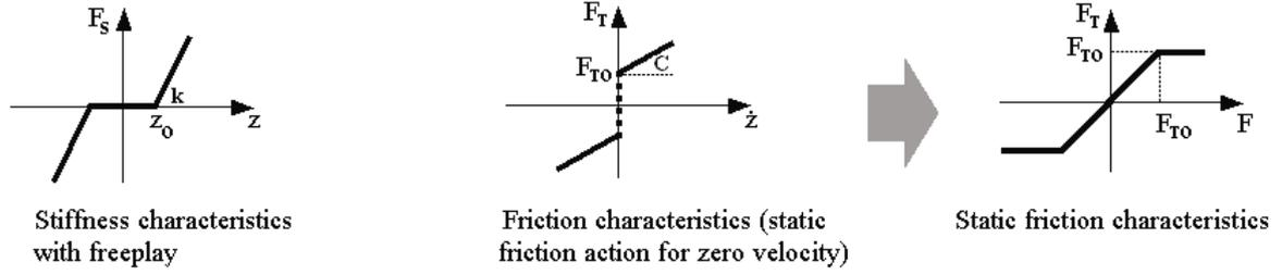
Fig. 2. Typical characteristics for freeplay and friction description. Here version when for kinetic and static friction force parameter  $F_{TK0} = F_{TS0} = F_{T0}$ . Notation:  $k$  – stiffness coefficient,  $C$  – viscous friction coefficient,  $F_{T0}$  – dry friction parameter,  $F_S$  – stiffness force,  $F_T$  – Friction force,  $z$  – displacement,  $\dot{z}$  – velocity,  $F$  – acting force
